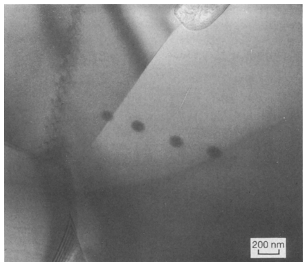
Figure 9 Transmission electron micrograph of a sample containing 1.4 at % Nb and sintered at 1420 °C for 8 h (Sr/(Ti + Nb) = 0.986). Dark spots are where EDS analysis were carried out. A TiO 2 second phase is observed in the upper right-hand side.
